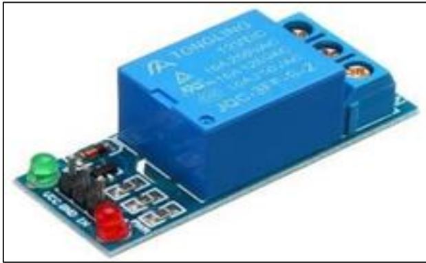
(b) Figure 13: (a) A 12V Water Pump; (b) Relay Module
